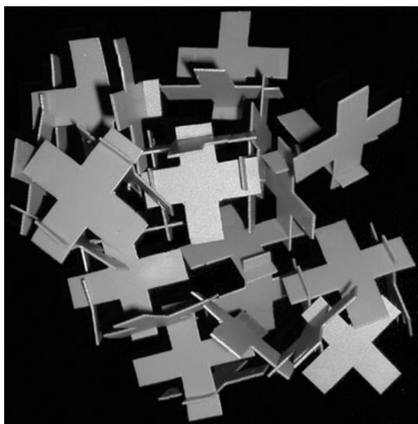
Figure 1. Simple three-dimensional model of the phthalocyanine-based microporous network polymer, with the aromatic macrocycles represented by cross-like shapes. The model helps to visualise the microporosity of the material, which is caused by the random and inefficient packing of the phthalocyanine units due to the rigid spirocyclic structure of the linking groups.
